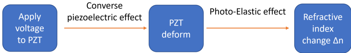
Figure 2. 7 Device working principle: converse piezoelectric effect and stress-optic effect.
