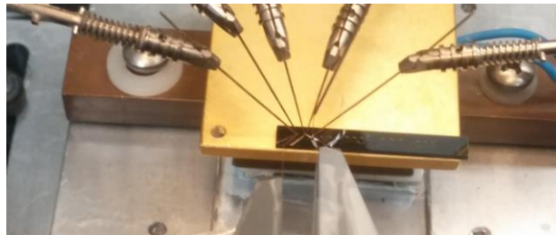
Fig. 30. Photograph of third-order filter being measured.
