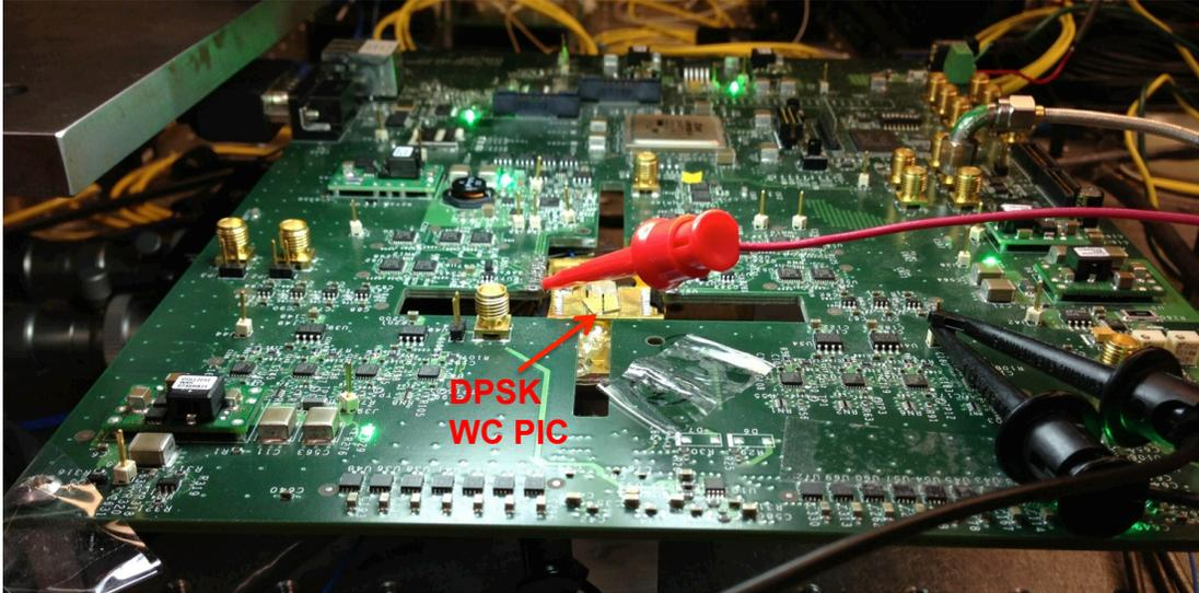
**Figure 5.25:** Photograph of the packaged DPSK wavelength converter PIC with FPGA controller board
