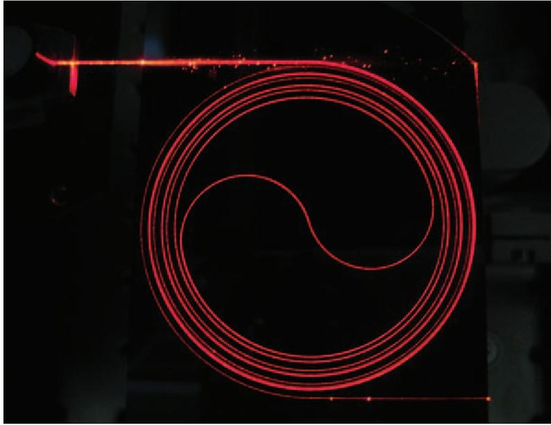
**Figure 1.1:** *An example of a 1 meter-long waveguide fabricated out of the glasses  $\text{Si}_3\text{N}_4$  &  $\text{SiO}_2$ , illuminated with a red laser from an optical fiber (top-left). The time-delay corresponds to about 5 ns.[12]*
