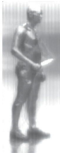
Figure 1.2: An individual holding a concealed weapon in a newspaper obtained at 94 GHz [6].
